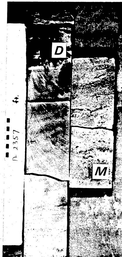
Figure 92. An incomplete cycle in the upper San Andres Formation Stone and Webster Engineering Corporation Detten No. 1 core, depth 2,357 ft. Mudstone insoluble residue in the top 10 cm of the core (M) formed by accumulation of insoluble components when halite was removed by the transgression that initiated the next cycle. Other evidence that halite was initially deposited is the abundant halite pseudomorphs after gypsum in the lower part of the core (H), indicating halite-saturated waters were important in earliest diagenesis, and the area of disturbed fabric at the top of the core (D) where removal of halite has altered fabrics like those seen in figure 90 at the anhydrite-halite contact.
