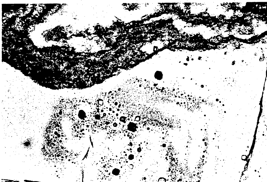
Figure 78. Photomicrograph of chevron halite truncated by a corrosion surface above which anhydrite (A) has been deposited. Width 3.25 mm, plane light, from unit 5 of the San Andres Formation, depth 1,438.0 ft, Stone and Webster Engineering Corporation Mansfield No. 1 core.
