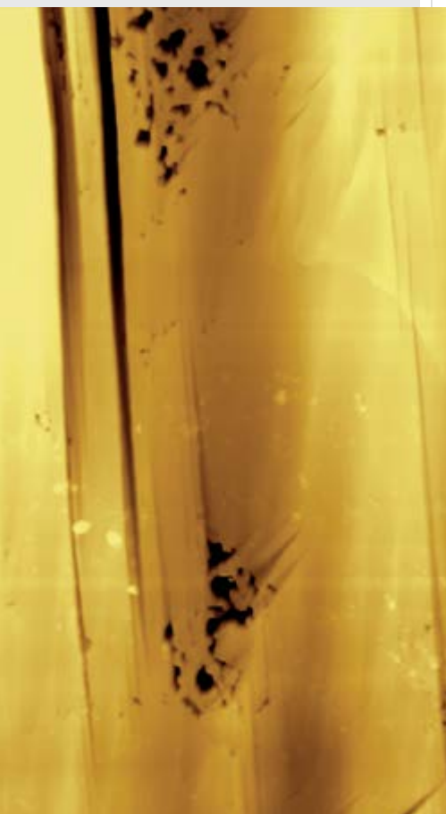
Darkest spots are nanopores on the surface of an ion-milled shale sample detected by an AFM.
