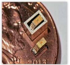
Advanced Energy Consortium's first-generation prototype multisensing microsystems shown here were developed by a team at the University of Michigan.
