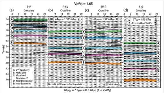
source. Two images (P-P and P-SV) are produced by the direct-P mode, and two images (SV-P and S-S) are produced by the direct-SV mode. A, B, C, and D are depth-equivalent horizons in the four image spaces. Data collected in the Midland Basin.
