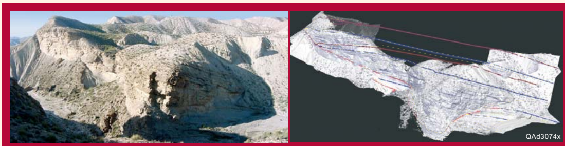
Photograph and laser-generated pointcloud of a Miocene-age deepwater canyon from the Tabernas Basin, southern Spain. The paleoflow direction is toward the observer. The canyon is 400 m wide and 60 m deep. Reservoir-grade sandstones and conglomerates occur within the erosional axis of the system and pass laterally into thin-bedded sandstones and shales toward the margins. Several high-frequency sequences defined by basal erosional surfaces (red horizons) and abandonment surfaces (blue) are mapped along the extent of the outcrop on the 3-D pointcloud data, producing a 3-D horizon and lithofacies interpretation similar to 3-D seismic data. The FRST research study uses outcrops like this as a basis for sophisticated 3-D geophysical modeling.
