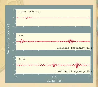
along Congress Avenue in Austin, Texas. The early event in each record is generated when the front wheels of the vehicles pass over a road bump; the later, larger event occurs when the rear wheels (carrying more weight) pass over the same bump. The time between the two events differs because the vehicles have different wheelbases and are traveling at differing speeds.
