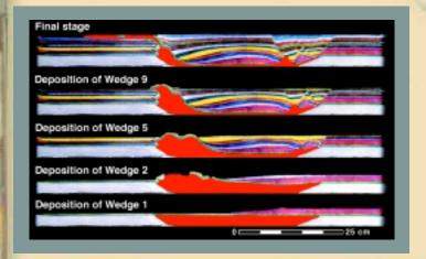
computer-controlled rigs to simulate structural styles while overhead photographs, serial sections, time-lapse videos, and CT scans assist in reconstructing and analyzing structural evolution. Modeling investigations include turtle structures, growth folds, diapir drag, strike-slip along allochthonous salt sheets, and extension above basement steps.
