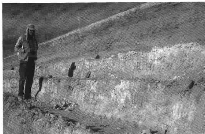
Bureau researcher examines calcic soil exposed in exploratory trench at the State's proposed site for a low-level radioactive waste disposal facility in Hudspeth County, Texas. The calcic soil is probably more than 100,000 to 300,000 years old. The exploratory trench was excavated in the fall of 1996 and is about 400 ft long and has a maximum depth of about 30 ft. The trench verified geologic relationships inferred from boreholes at the site. Photo by Jay A. Raney.
