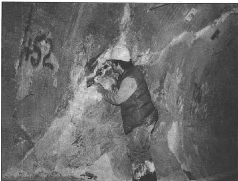
Bureau scientist examines a mineralized fault in the lower Austin Chalk exposed in the wall of the Superconducting Super Collider (SSC) tunnel in Ellis County, Texas. Mapping of numerous fractures in the tunnel and in surface excavations is part of a larger, comprehensive study of ground-water movement at the SSC site. Photograph by Kenley C. Schroeder.
