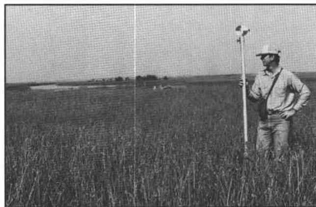
Bureau researcher conducting an elevation survey of a brackish-water marsh on the Trinity River delta, Chambers County, Texas. This data-gathering is designed to help determine historical land loss or gain, sedimentation rates, and changes in emergent vegetation in major fluvial-deltaic areas along the Texas Gulf Coast.
