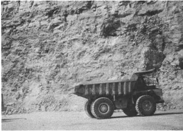
Edwards Limestone (Lower Cretaceous) quarry in Balcones Fault Zone area. The Edwards is an important calcareous resource for Texas cement plants.
