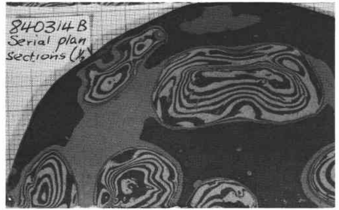
Horizontal section through a centrifuged model showing the internal structure of diapirs. The zebra stripes within the diapirs were originally horizontal and uniformly thick. Experiment performed at the University of Uppsala, Sweden.
