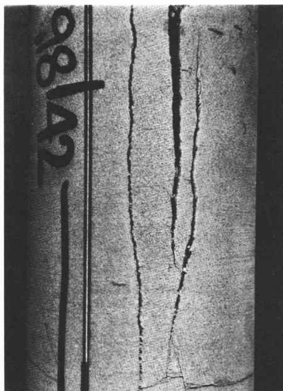
Natural, open extension fracture in Travis Peak sandstone core from a depth of 9,842 ft in the second Staged Field Experiment well in East Texas. Such open fractures can enhance reservoir permeability in low-permeability gas sandstones. Maximum width of this fracture is 0.2 inch.
