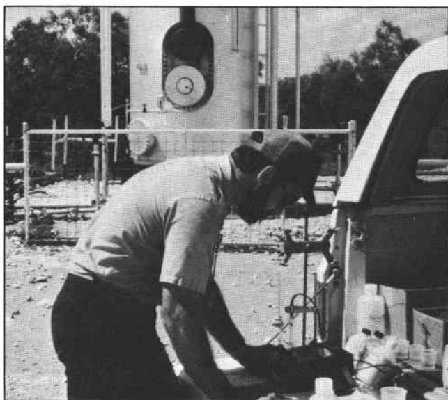
Research Associate Alan Dutton tests alkalinity and pH of an oil field brine near San Angelo as part of an investigation for the Railroad Commission of Texas to determine sources of salt-water pollution in western Tom Green County.
