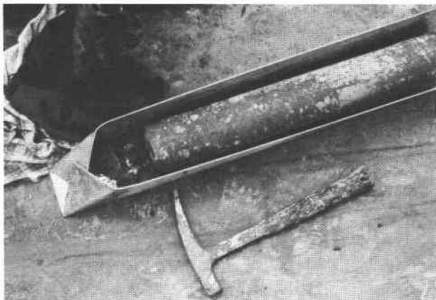
Aligning the orientation equipment as the core barrel is assembled, catching the core in trays on the rig floor, and preliminary examining of core, here showing a conglomerate, for the first Travis Peak well studied in cooperation with an operator on the GRI tight gas sandstone project.
