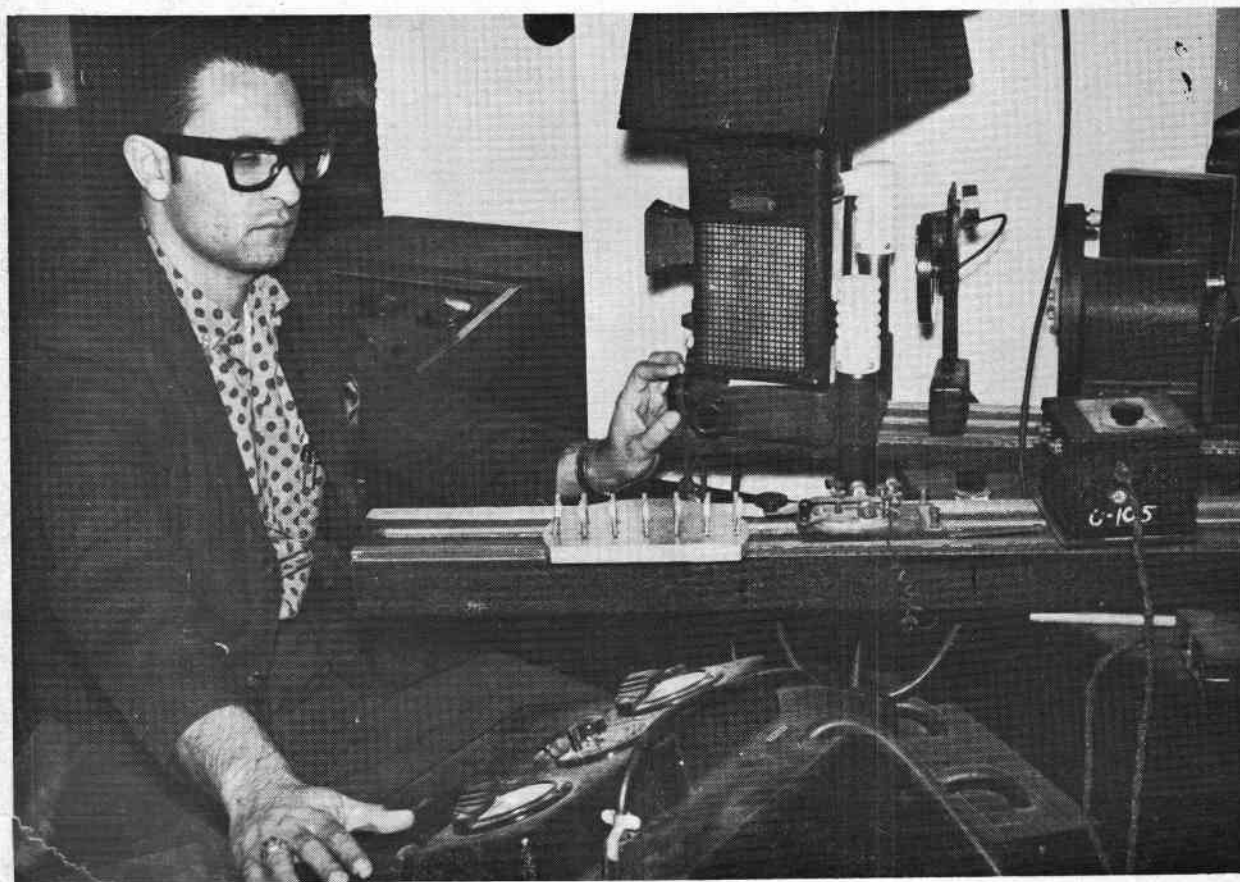
The ARL 1.5 meter emission spectrophotograph in operation at the Mineral Studies Laboratory. The operator, Fernando D. Cortes, is a chemical engineering student employed as a laboratory assistant by the Bureau.
