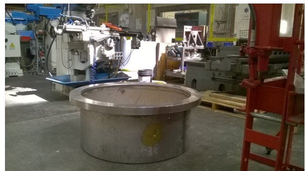
Body of stainless steel tank (1-m diameter and 0.5-m height) for performing laboratory harmonic well testing
