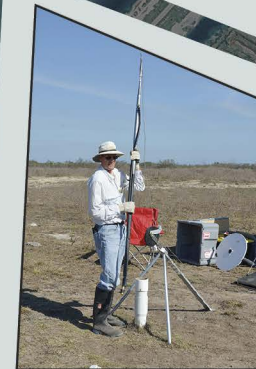
Borehole probe being lowered into a water well to measure the electrical conductivity of the shallow subsurface during geologic mapping on the Texas Coastal Plain.
