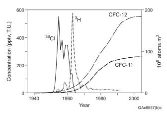
Figure 2. Input functions for historical tracers, including <sup>3</sup>H, <sup>36</sup>Cl, CFC-11 and CFC-12 (<sup>3</sup>H data from Ottawa, Canada; <sup>36</sup>Cl data, Phillips 2000; CFC data, http://water.usgs.gov/lab/cfc/background/air\_curve.html).
