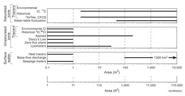
Figure 7. Spatial scales represented by various techniques for estimating recharge. Point-scale estimates are represented by the range of 0 to 1 m.
