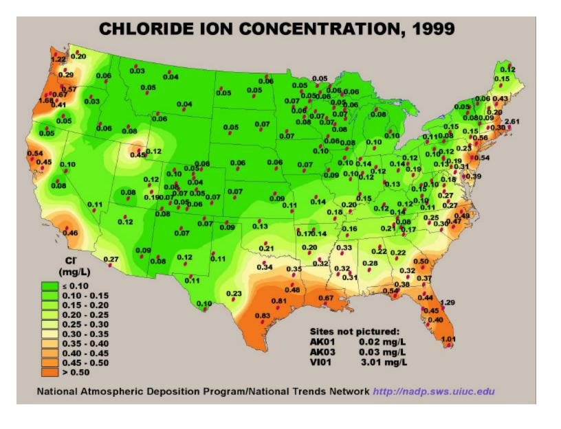
Figure 14. Wet chloride fallout in precipitation from the National Atmospheric Deposition Program.
