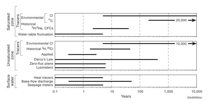
Figure 8. Time periods represented by recharge rates estimated using various techniques. Time periods for unsaturated-and saturated-zone tracers may extend beyond the range shown.
