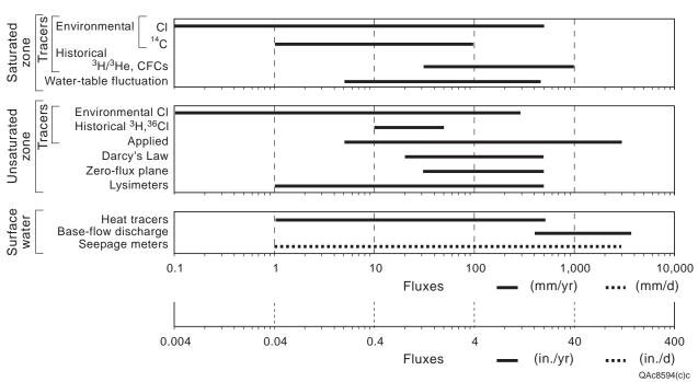
Figure 6. Range of fluxes that can be estimated using various techniques.
