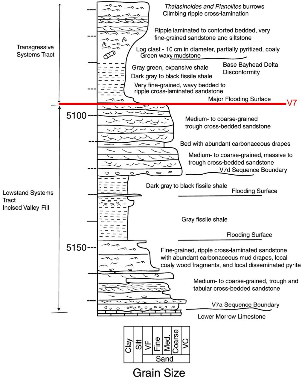
Figure 12. Sedimentological descriptive log for No. 3 Schneider 34-1 well illustrating facies stacking patterns for a “downdip facies tract.” See Bowen and Weimer’s (2003) figure 7a for accompanying core photos. Note V7 “regional” flooding surface highlighted in red. Note change from lowstand to transgressive systems tract that will not be overly apparent on wireline logs.
