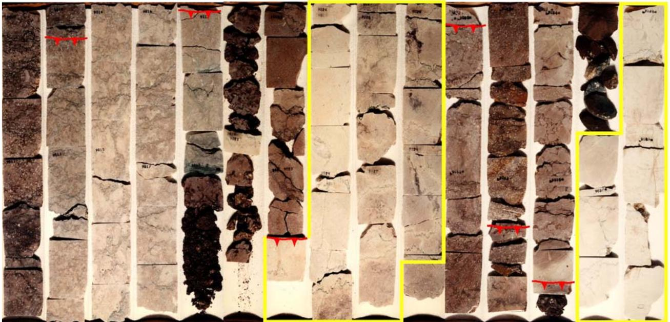
Figure 38. Middle Cisco exposure style 4 core photographs, core description, and isotopic profiles (after Saller and others, 1999a). Textural alteration is extensive compared with that of the underlying interval illustrated in figure 37. Cycle tops indicated in red on core photographs. Upper reservoir interval (yellow outline) thickness is approximately 6 ft, whereas lower is approximately 10 ft (not all depicted).
