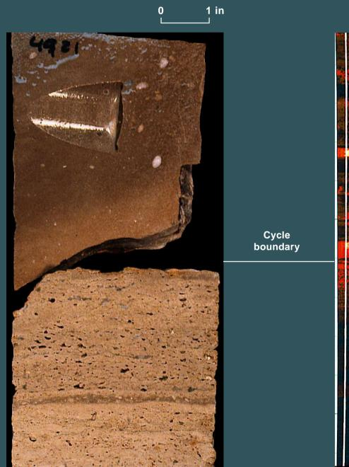
20. Paired core and FMI log image: upper San Andres. FMI has very high resolution that can be used to discriminate even the finest scale cycles and facies successions. Note: Core depths are about 5 ft higher than log.
