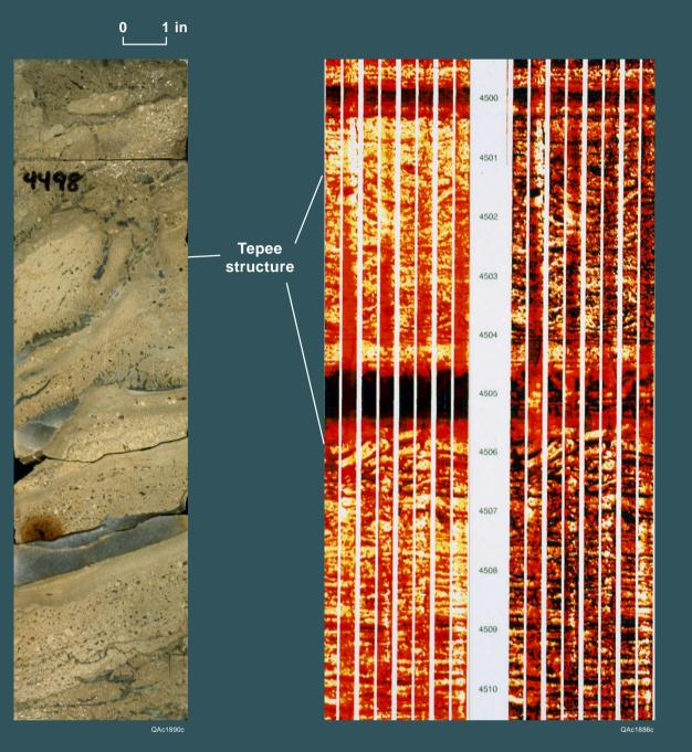
17. Paired core photograph and FMI log image: upper San Andres tidal-flat rocks. Tidal-flat facies are characterized on FMI by thin laminated character. Note tepee structure.
