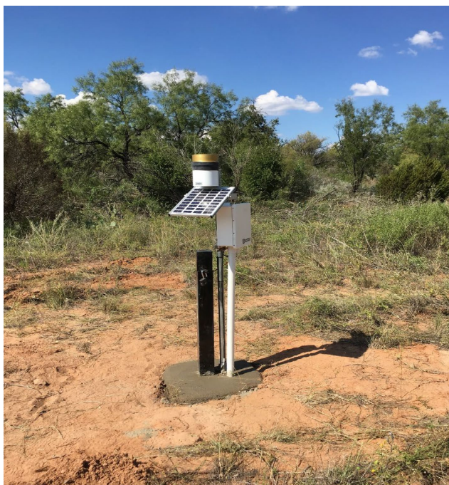
Figure 2. Representative monitoring site, including solar panel, rain gage, and data-logger. Site shown is enclosure at DMF1 middle terrace well.
