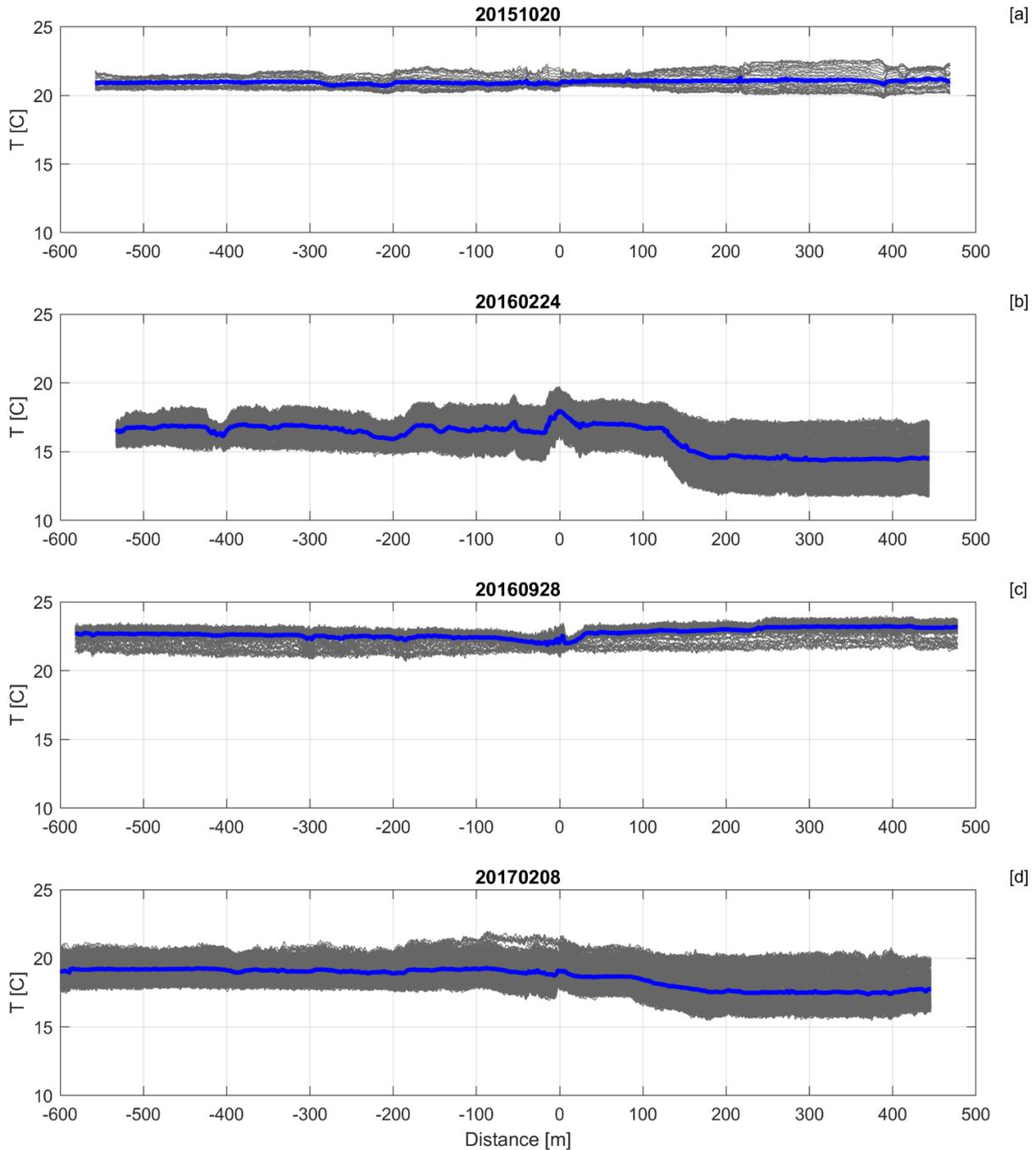
**Figure 26. Instream distributed temperature sensing fiber optic measurements for [a] October 2015, [b] February 2016, [c] September 2016 and [d] February 2017. Gray lines indicate 6-minute measurements aggregated into mean (blue) for the measurement period. The origin distance (0 m) begins on the rock ledges heading ~ 400 m upstream and ~ -600 m downstream.**
