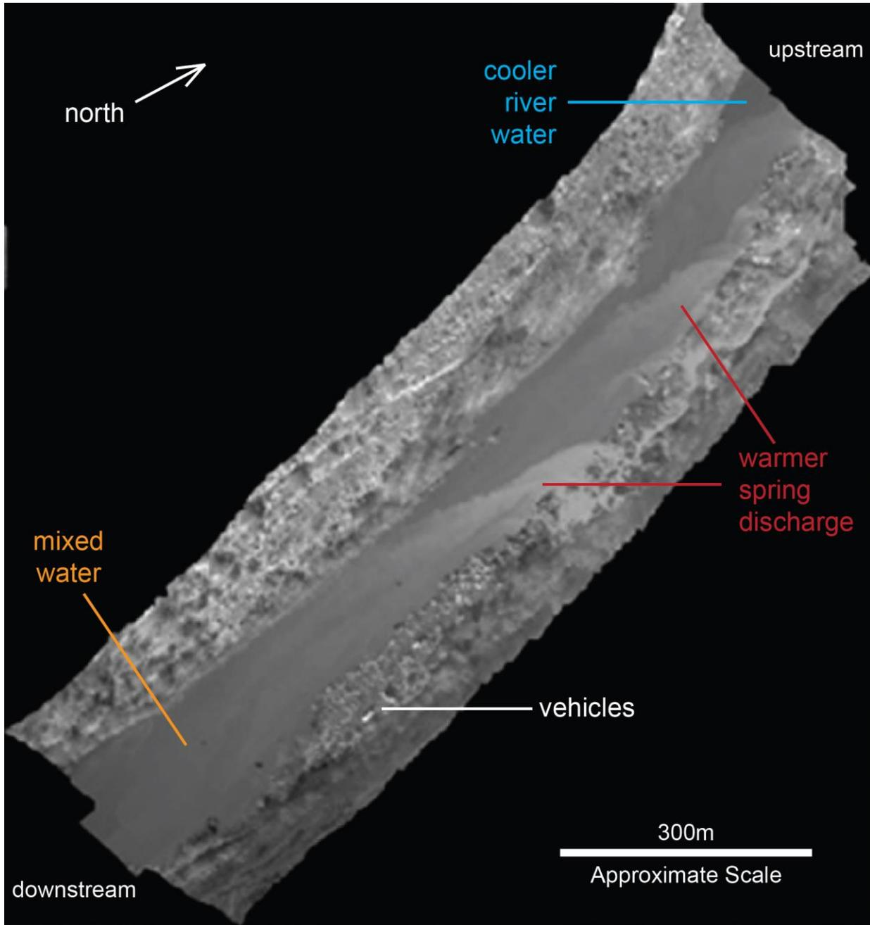
**Figure 28. Thermal infrared UAS imagery of Devils River and spring run water relative surface temperature (lighter gray=warmer)**
