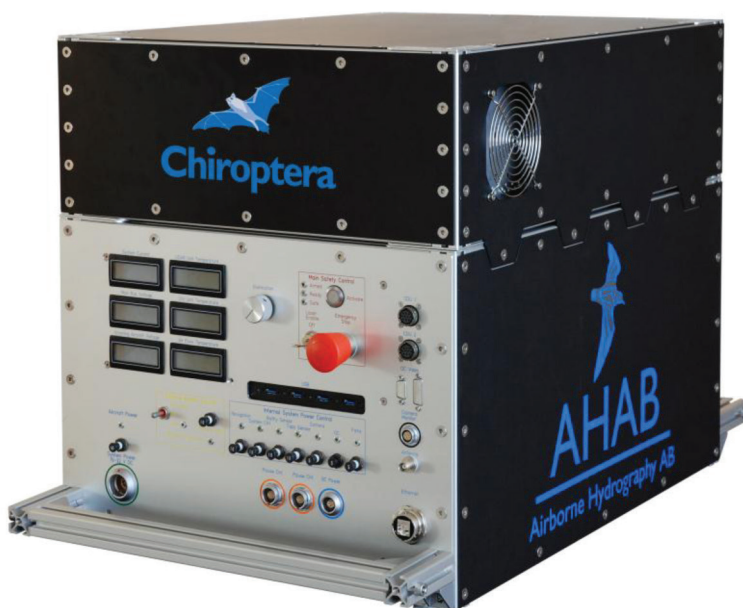
Figure A1. The Bureau's Chiroptera airborne lidar and imagery system. The system was built for the Bureau by Airborne Hydrography AB and delivered in July 2012.
