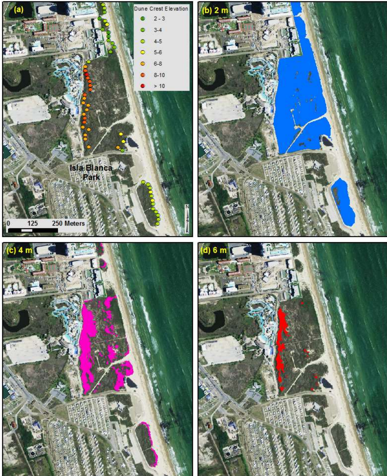
Figure 28. Developed segment of South Padre Island with seawall (a) showing maximum dune crest elevations. Areas of threshold elevations greater than (b) 2 m, (c) 4 m, and (d) 6 m. This area north of Brazos Santiago Pass and Isla Blanca Park is only section with mature foredune with dune crests greater than 6 meters.
