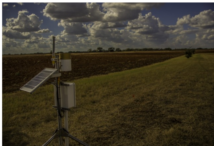
A TxSON Soil moisture sensor. Credit: Richard Casteel.
