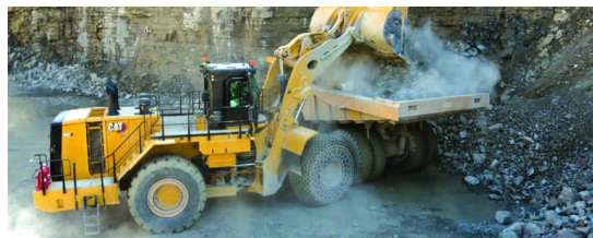
Payload Overload Prevention on the new 992 helps prevent an overloaded bucket from being raised to full truck height. It either slows or stops the action when a payload threshold is exceeded. (Photo: Caterpillar)
