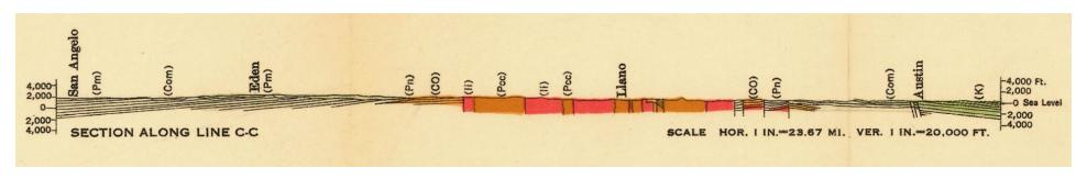
**[top]** Four lines show regional elevations and subsurface formations, the longest stretching from the Panhandle to the Gulf Coast. **[bottom]** A detailed view of the line stretching from San Angelo to Austin.
