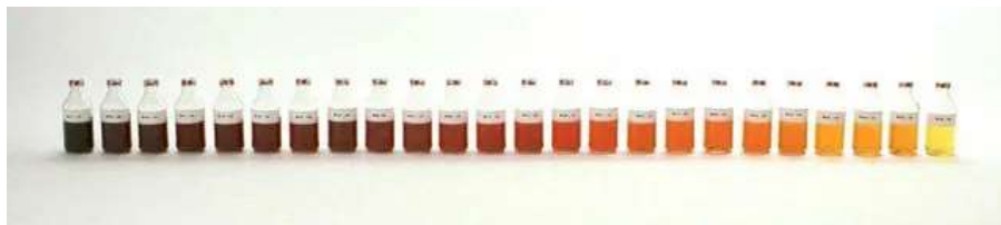
Color variations of a crude oil column from a single connected reservoir. Courtesy D. McKinney, H. Elshahawi, Shell Oil Co. ( ResearchGate )
