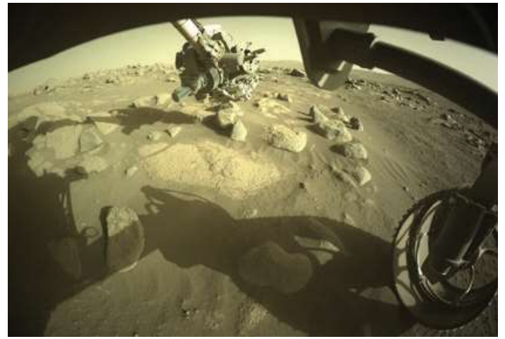
Left: Ingenuity Flight 4- April 30, 2021 (Sol 69). Ingenuity is left of center with a spectacular delta outcrop in the distance. Right: Mars Perseverance Rover front right HazCam image Sol 79/May 11, 2021. Visible in the image is the rover's right front wheel, and the turret at the end of the instrument arm carries scientific cameras, mineral and chemical analyzers for studying Mars geology. Instruments on the turret are SHERLOC, WATSON, PIXL, and the geology sample drill. Image courtesy of NASA/JPL-Caltech.
