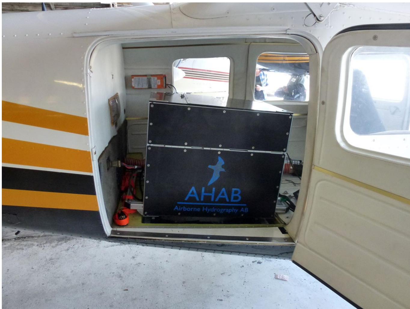
The Bureau's Chiroptera airborne lidar system installed in an aircraft for a coastal survey. (Credit: Bureau of Economic Geology)
