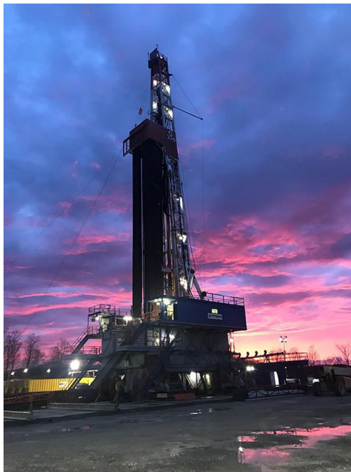
A Patterson-UTI rig drilling on the Northeast Natural Energy MSEEL Boggess Pad outside of Core, West Virginia. Six 10,000 ft laterals were drilled and instrumented. Completions operations are under way. Source: MSEEL.
