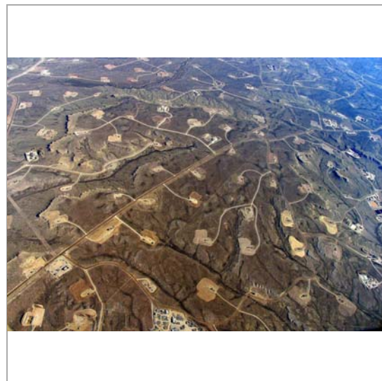
IMAGE: THIS IS AN AERIAL VIEW OF HYDRAULIC FRACTURING OPERATIONS ACROSS THE JONAH FIELD, A LARGE NATURAL GAS FIELD IN WYOMING. view more >
