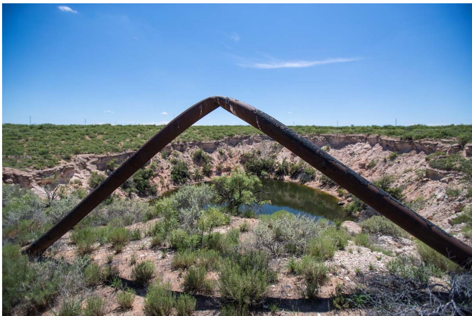
A twisted pipeline stretches above Wink Sink No. 1, showing the force of the collapse of tons of dirt. RAFAEL AGUILERA
