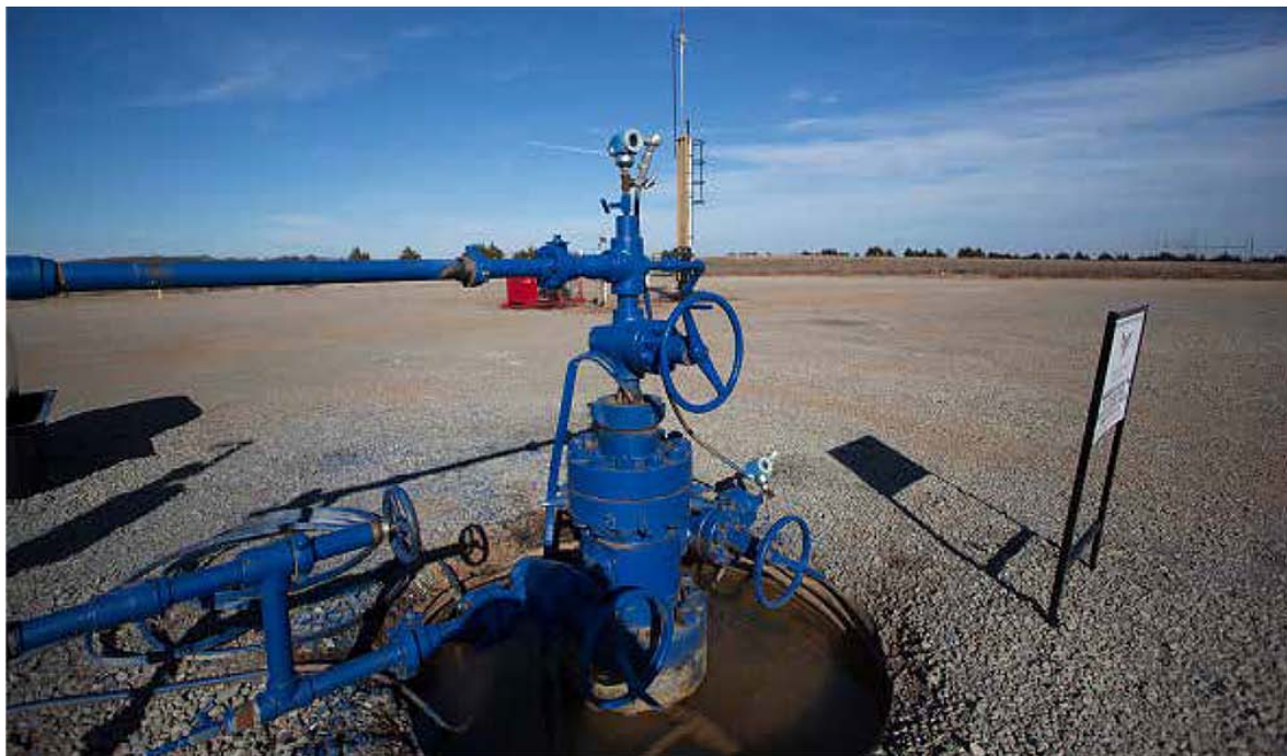
A wellhead in Coyle, Okla., pumps wastewater into a deep, underground rock formation for permanent disposal. Thousands of disposal wells operate across the state.
