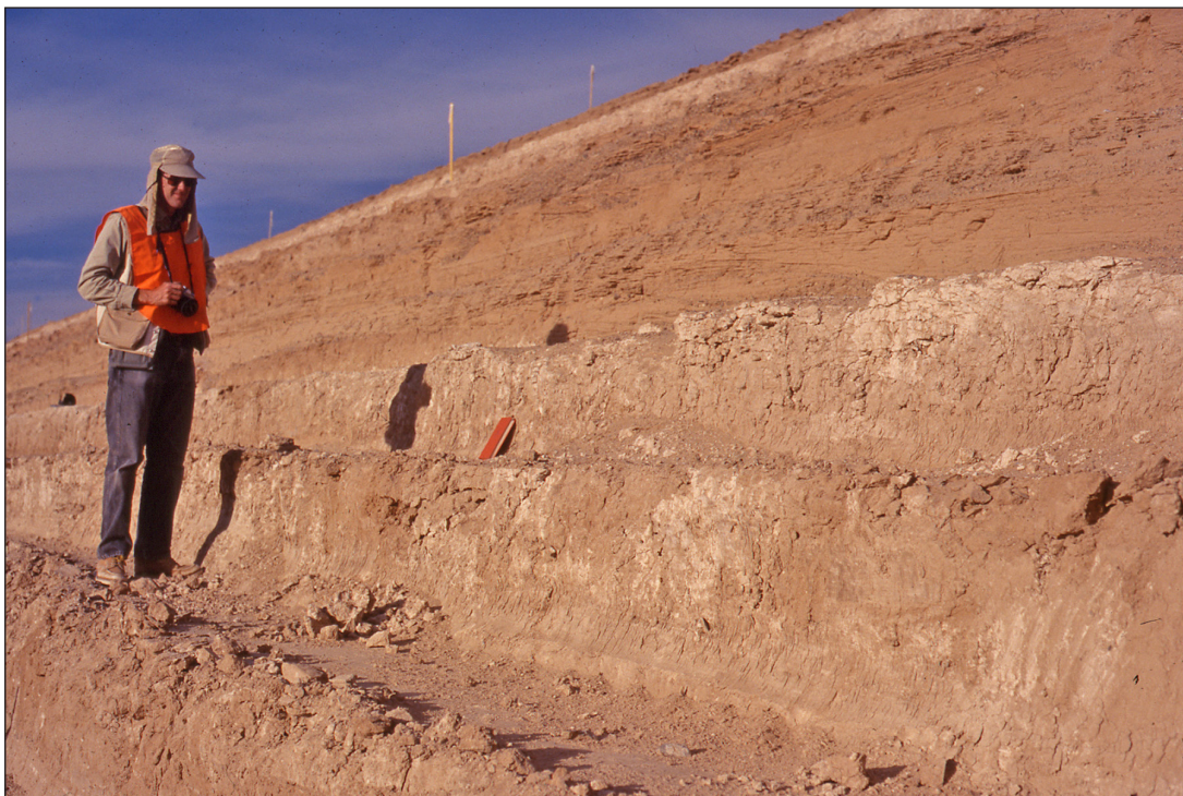
Eddie examining a trench across a fault for the Low Level Radioactive Waste Disposal Project near Sierra Blanca, Texas. Photograph by Jay Raney.
