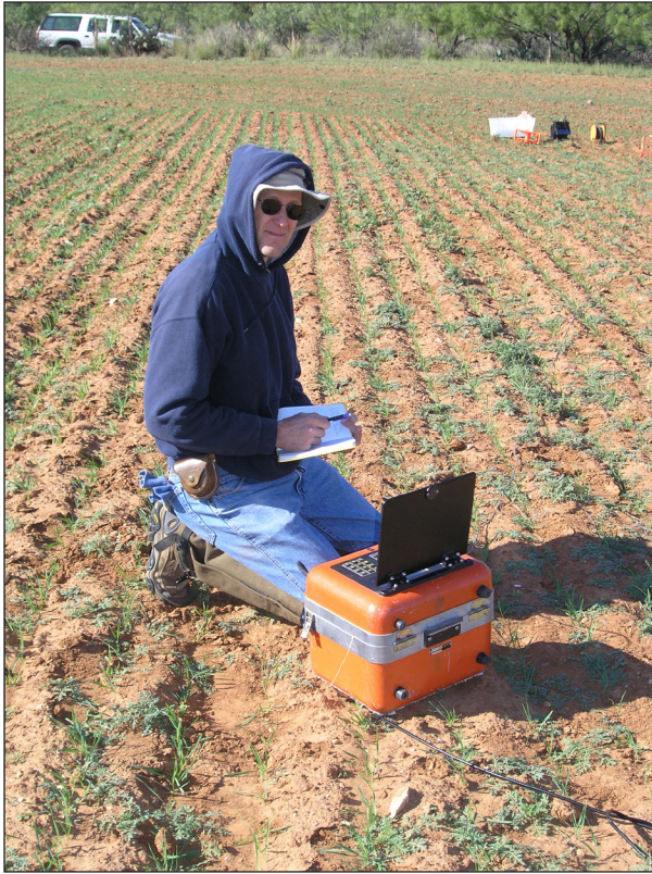
Eddie reviewing time-domain EM data over a salinity plume in the Wendkirk Oil Field adjacent to the Colorado River, Coke County, Texas, November 2006. Photograph by Jeff Paine.
