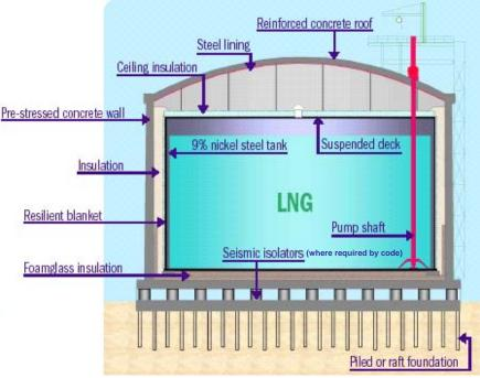
Figure 13. Conceptual Design of Storage Tanks
