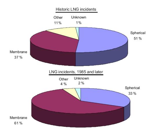
Figure 27. LNG incidents before and after 1985 by ship type
