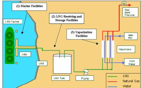
Figure 8. Typical LNG Receiving Terminal/Re-gasification Facility
