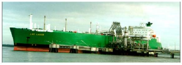
Figure 16. LNG Lagos - Membrane Type LNG Carrier
