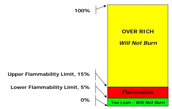
Figure 3. Flammable Range for Methane (LNG)
