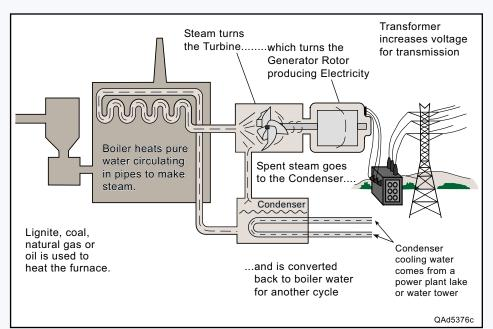
Figure 8. Steam Turbine Electric Power Plant
