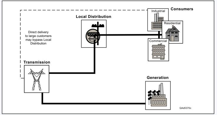
Figure 2. Basic Electric Power System
