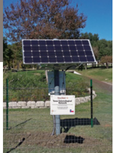
TexNet seismometers placed throughout the state, like this one in Dallas, monitor seismic activity across Texas.
