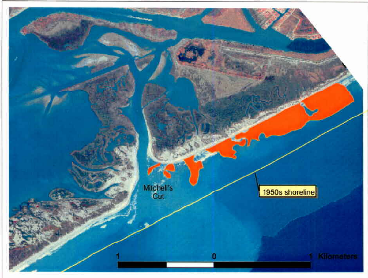
Figure 27. Loss of estuarine marsh since the 1950's due to erosion of the northeast end of Matagorda Peninsula at Mitchell's Cut. Loss shown in red. Erosion rates in this area are as high as 8m/yr (27 ft/yr). Photograph taken in 2001 by ALS, Inc.
