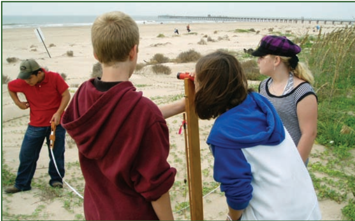
Students survey a shore-normal beach profile from the foredunes to the waterline using a sighting level.
