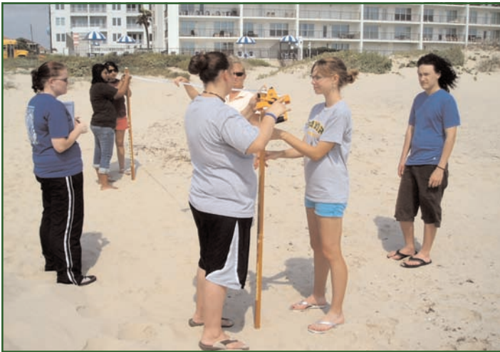
Measuring the beach profile to compare to past results on South Padre Island.
