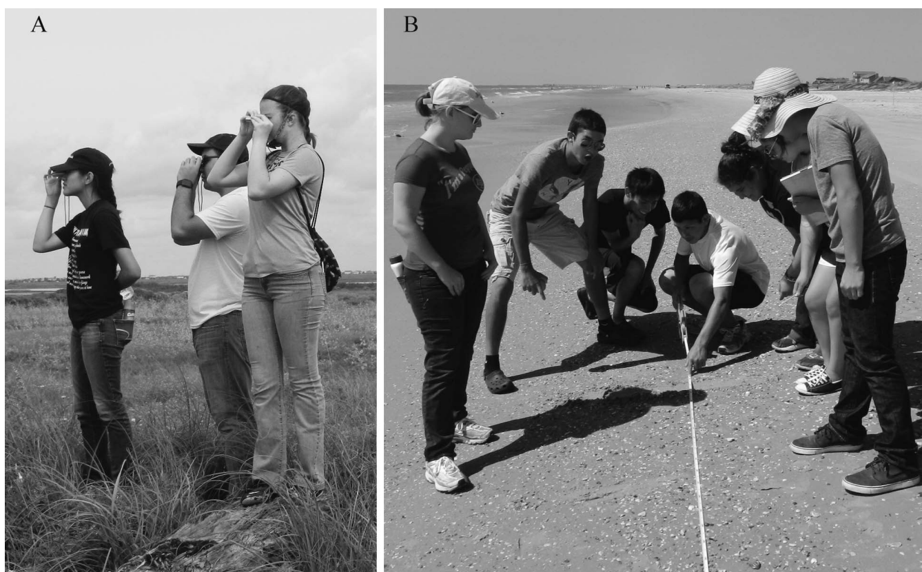
Figure 3. Students (A) using a sighting compass to measure dune orientation, and (B) measuring how far along the shoreline the float (an orange) drifted to determine longshore current speed and direction.
