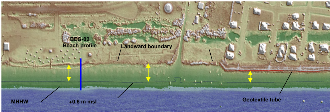
Figure 10. Lidar topographic relief image of Galveston Island State Park and Pirates Beach subdivision. Note difference in beach width between the natural beach and that in front of the subdivision.
