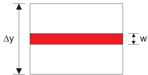
Figure 5. Grid cell representation of a fracture patch, showing the cell dimension and fracture aperture.
