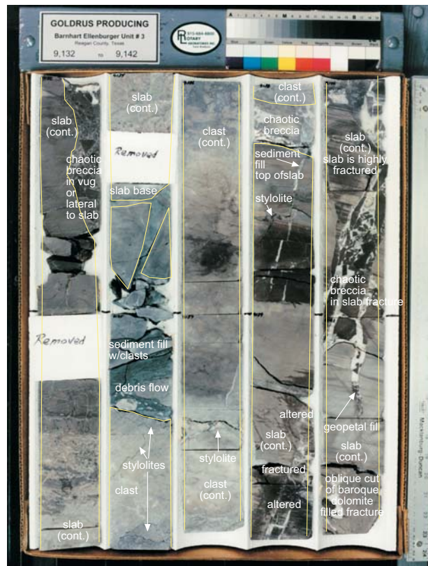
Large deformed blocks with crackle breccia overprint.
