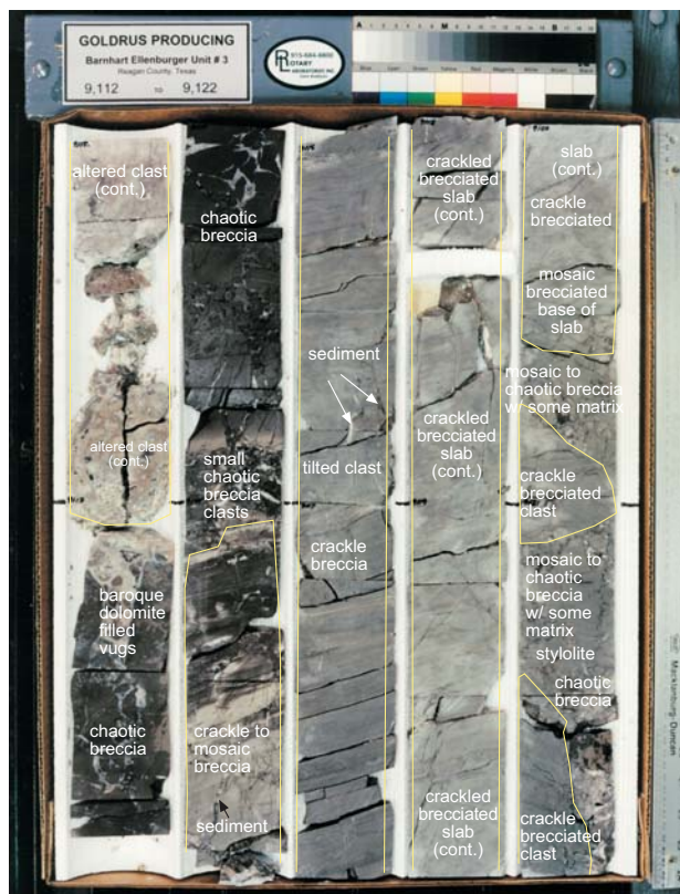
Large deformed blocks with crackle breccia overprint.
