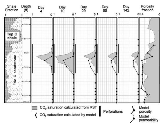
Figure 1. RST logs collected during the Frio Brine Pilot test. CO<sub>2</sub> saturation at the observation well is compared with modeled changes in saturation per layer plotted at layer midpoint.
