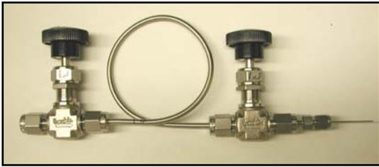
Figure 2. Sample loop (1 mL) used to inject fluid samples into glass vials for transport and analysis
