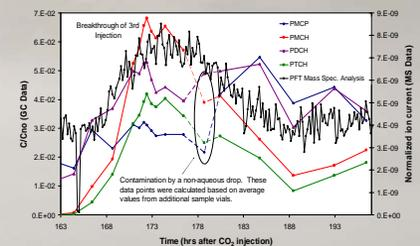
Figure 6: C/C<sub>no</sub> data from GC and MS analyses for all PFTs during the third breakthrough.
