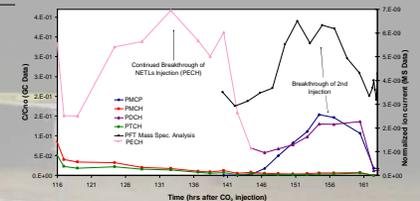
Figure 5: C/C<sub>no</sub> data from GC and MS analyses for all PFTs during the second breakthrough. PECH is represented by the pink curve and was the PFT introduced by a collaborating party.
