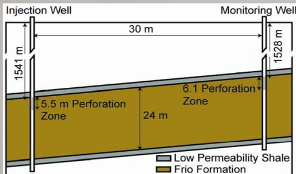
Figure 2: Cross section of the injection and monitoring well configuration and orientation of the Frio Formation (not to scale).
