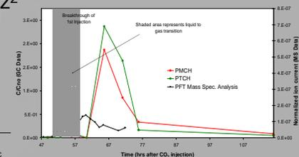
Figure 4: C/C<sub>no</sub> data from GC and MS analyses for all major injected PFTs during the first breakthrough. Shaded area represents the transition from liquid to gassy samples.
