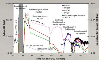
Figure 3: C/C<sub>no</sub> data from GC and MS analyses of all PFTs for all breakthroughs. Shaded area represents the transition from liquid to gassy samples. Hours 72-103 represent stand down time.
