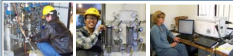
Fig. 6. High-frequency fluid sampling using the U-tube sampler (Freifeld et al., 2005). Samples were analyzed on-site using a mass spectrometer.
