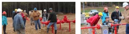
Fig. 4. CO 2 injection began at the DAS December 1, 2009, at a rate of 175 kg/min, with a step up to 350 kg/min.
