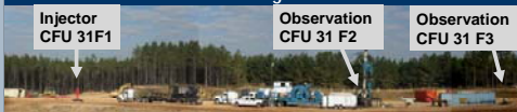
Fig. 2. Photo of the DAS (detailed area of study), a closely spaced well array to examine flow in a complex reservoir (by Tip Meckel and Susan Hovorka).
