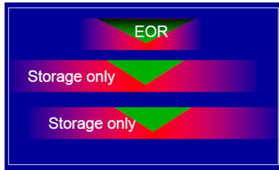
Figure 6. Large volumes of non-productive brine formations lie below many CO<sub>2</sub> EOR targets. The concept of using them to increase the sequestration volume accessed via EOR is called stacked storage.
