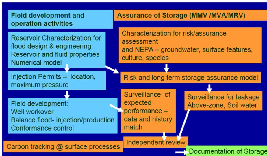
Figure 5 Draft plan linking commercial surveillance for CO<sub>2</sub> EOR with monitoring to document permanence of sequestration.
