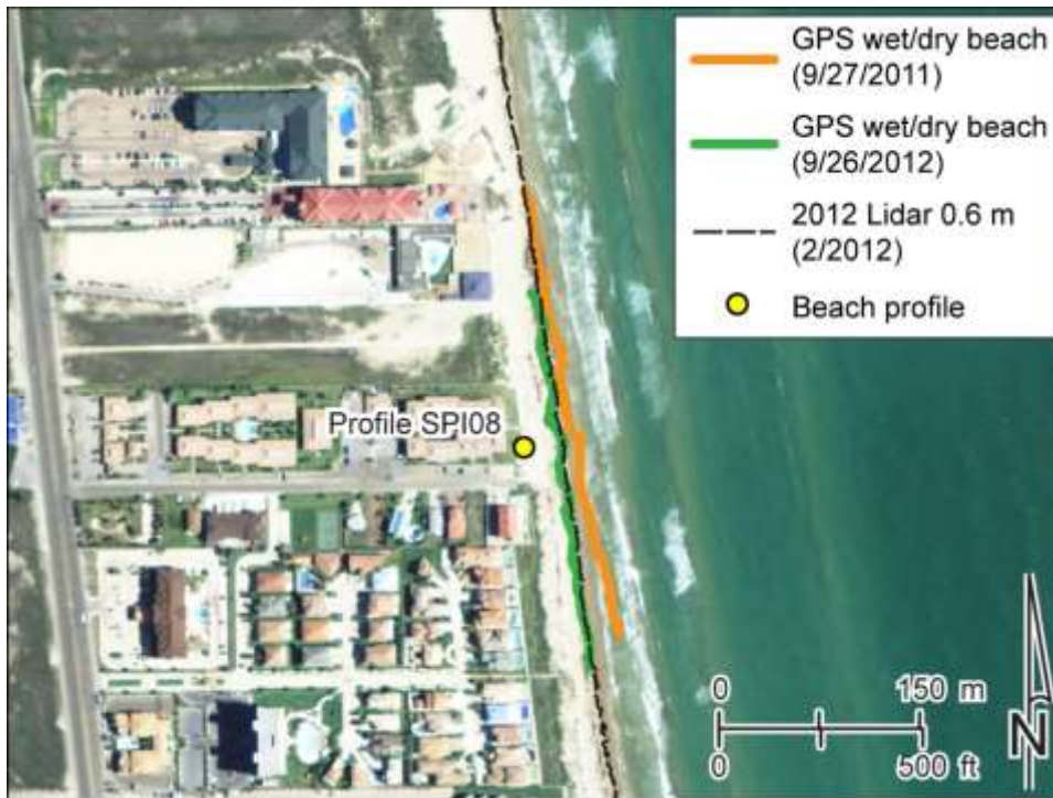
Figure 14. Shoreline position comparison at South Padre Island site SPI08. Shorelines include the wet-beach/dry-beach boundary mapped on September 27, 2011, and September 26, 2012, by THSCMP students using GPS and the shoreline proxy extracted from airborne lidar data acquired in February 2012. Shorelines are superimposed on NAIP imagery acquired on April 23, 2012. From Paine and others (2014).
