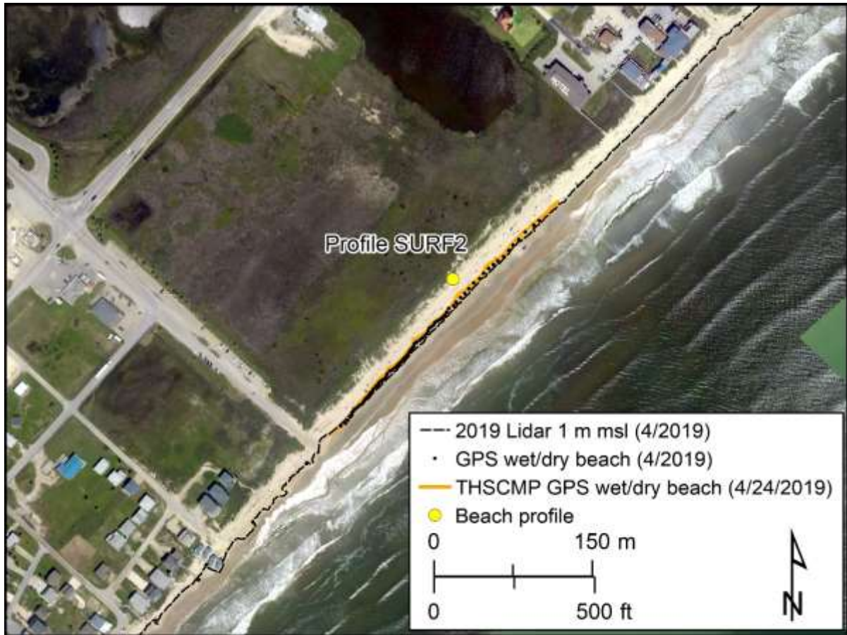
Figure 15. Shoreline position comparison at Surfside Beach site SURF2. Shorelines include the wet-beach/dry-beach boundary mapped on April 24, 2019, by THSCMP students and Bureau staff using ground GPS and the 1 m (3.3 ft) above mean sea level shoreline proxy extracted from airborne lidar data acquired in spring 2019, superimposed on 2019 Bureau imagery. From Paine and Caudle (2020).
