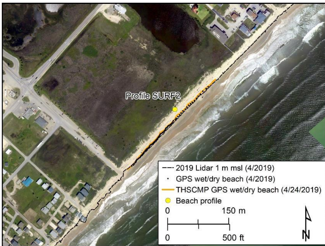
Figure 14. Shoreline position comparison at Surfside Beach site SURF2. Shorelines include the wet-beach/dry-beach boundary mapped on April 24, 2019, by THSCMP students and Bureau staff using ground GPS and the 1 m (3.3 ft) above mean sea level shoreline proxy extracted from airborne lidar data acquired in spring 2019, superimposed on 2019 Bureau imagery. From Paine and others (2021).
