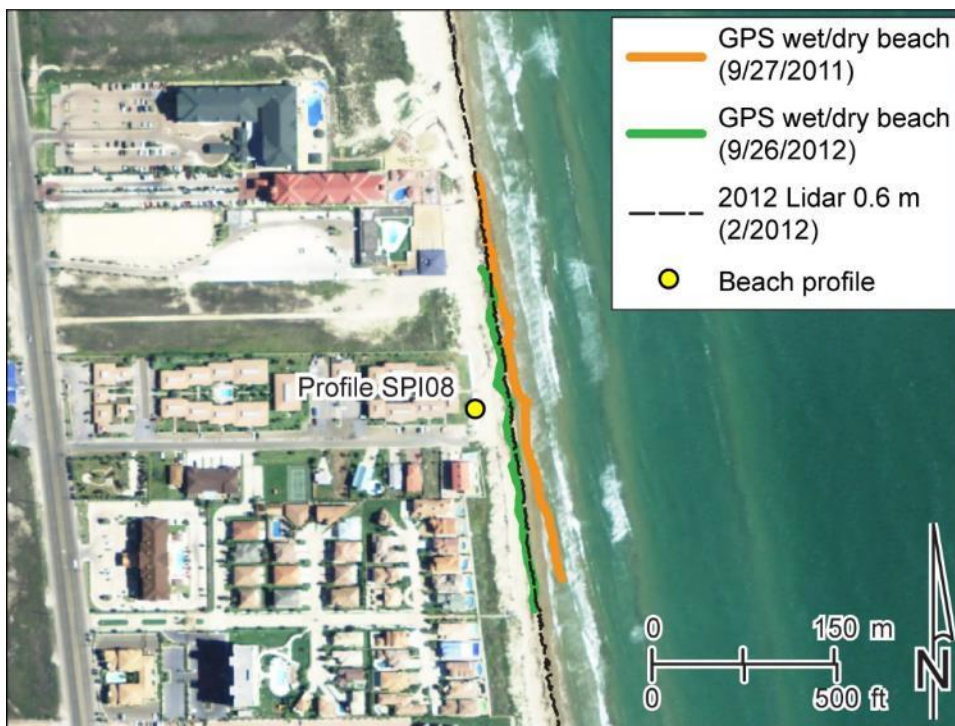
Figure 13. Shoreline position comparison at South Padre Island site SPI08. Shorelines include the wet-beach/dry-beach boundary mapped on September 27, 2011, and September 26, 2012, by THSCMP students using GPS and the shoreline proxy extracted from airborne lidar data acquired in February 2012. Shorelines are superimposed on NAIP imagery acquired on April 23, 2012. From Paine and other (2014).
