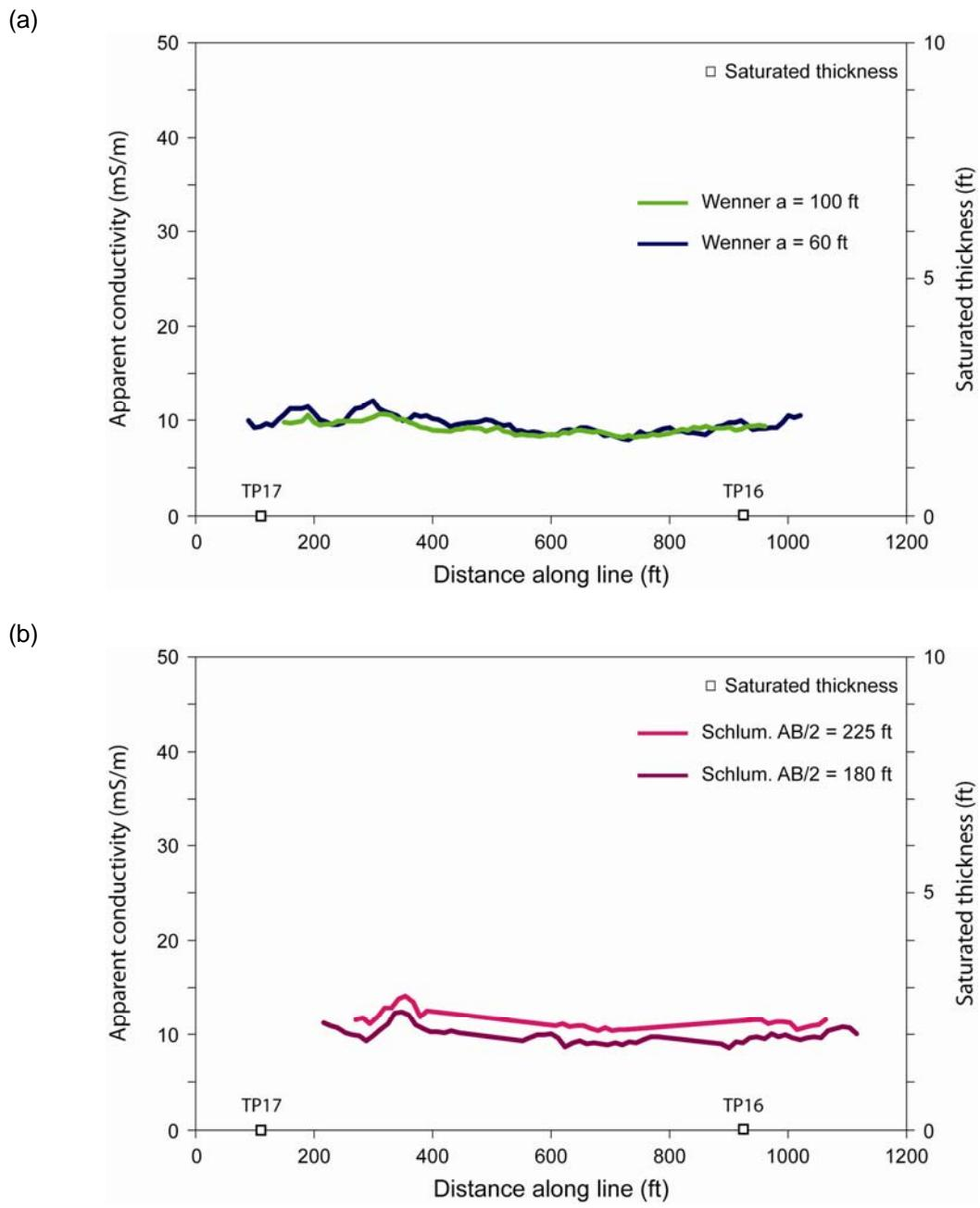
Figure 2. Comparison of apparent conductivity and water saturation along Line A.
