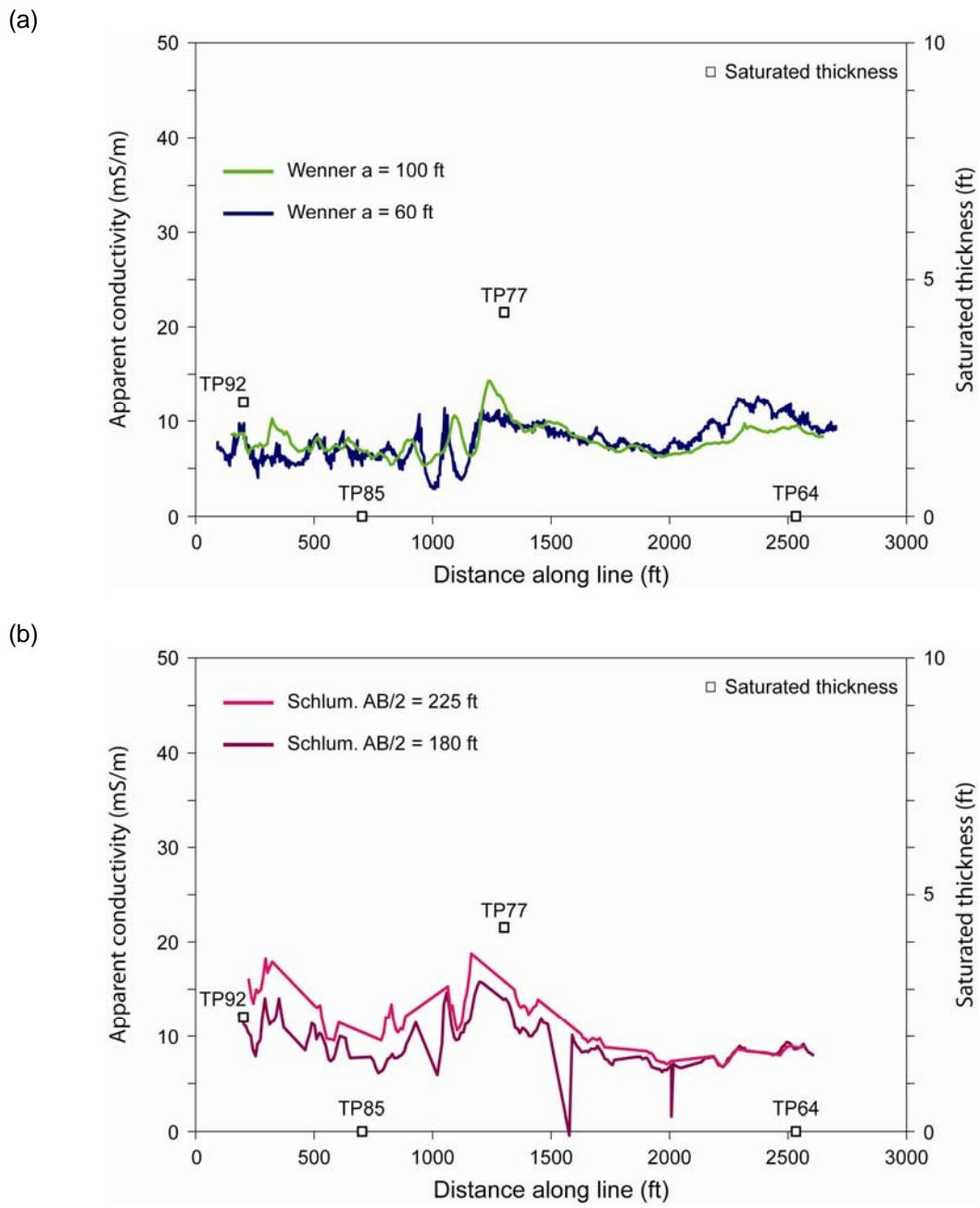
Figure 5. Comparison of apparent conductivity and water saturation along Line D.
