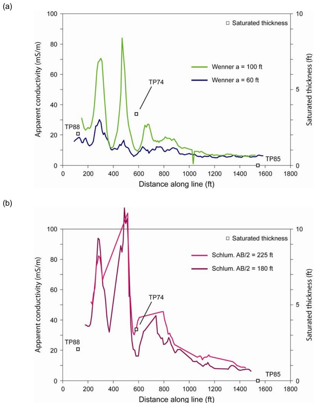
Figure 4. Comparison of apparent conductivity and water saturation along Line C.
