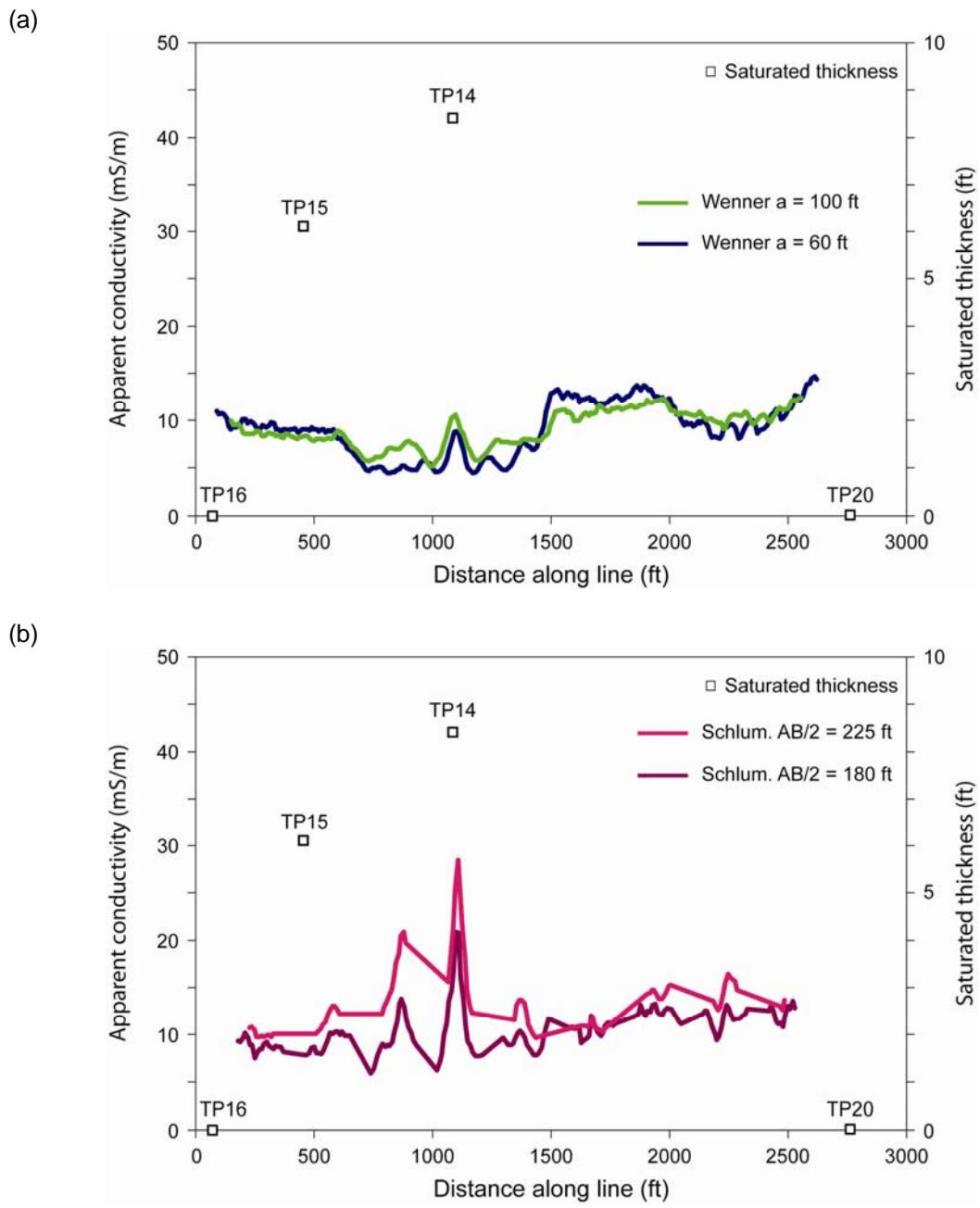
Figure 3. Comparison of apparent conductivity and water saturation along Line B.
